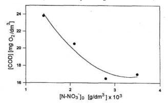
Fig. 2. The effect of the concentrations of nitrates on COD reduction in waste B (after rye-molasses processing, undiluted,  $37^{\circ}$ C).
