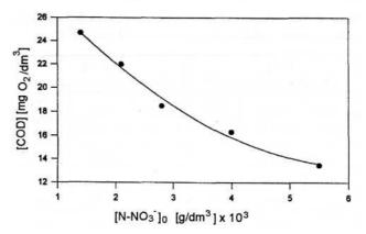
Fig. 1. The effect of the concentration of nitrates on COD reduction in waste A (after molasses processing, dilution 1:1, 37°C).
